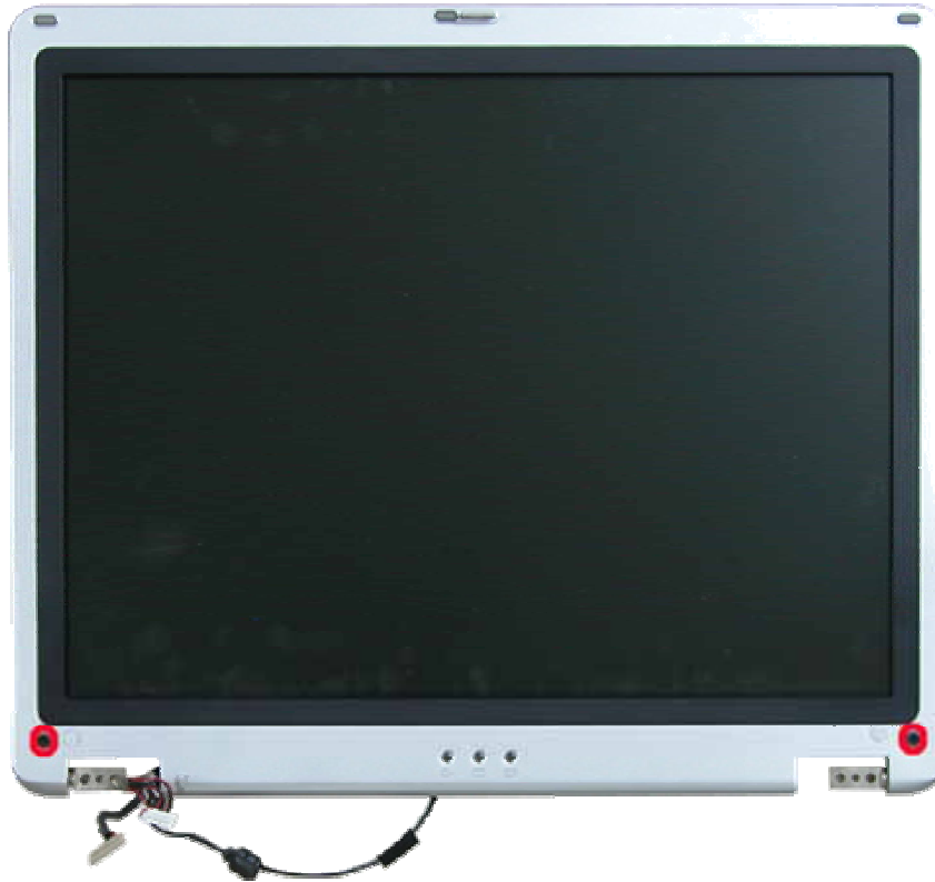
Fig. 25 Removing the rubber covers & screws on the LCD Module
